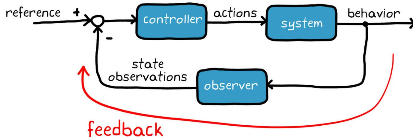
With feedback control systems, the controller uses state observations to improve performance and correct for random disturbances and errors. Engineers use that feedback, along with a model of the plant and environment, to design the controller to meet the system requirements.
