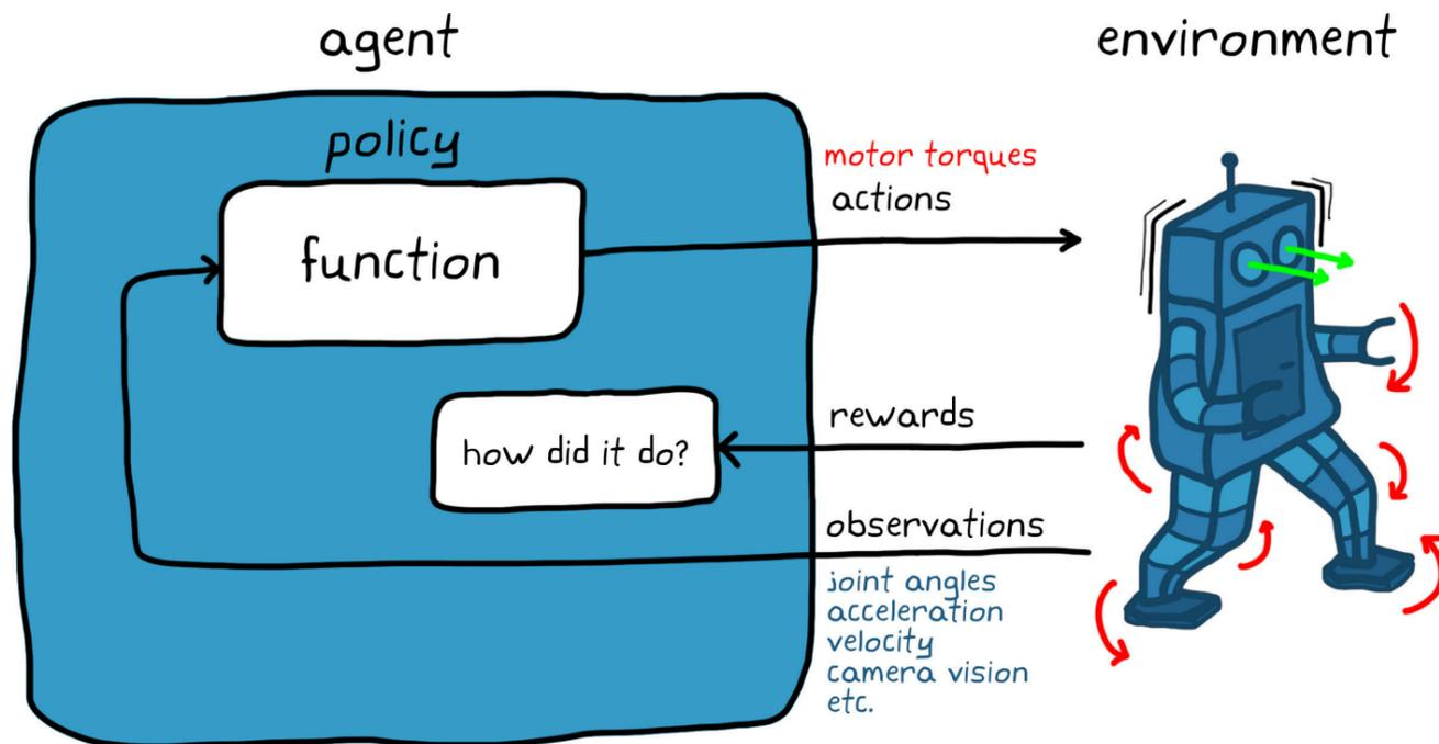
In the walking robot example, the observations would be the angle of every joint, the acceleration and angular velocity of the robot trunk, and the thousands of pixels from the vision sensor. The policy would take in all of these observations and output the motor commands that will move the robot's arms and legs.
