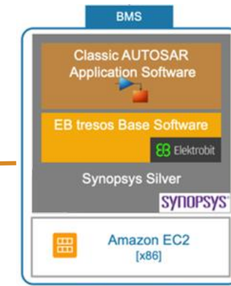
Virtual ECU running on a POSIX containerized environment on EC2
