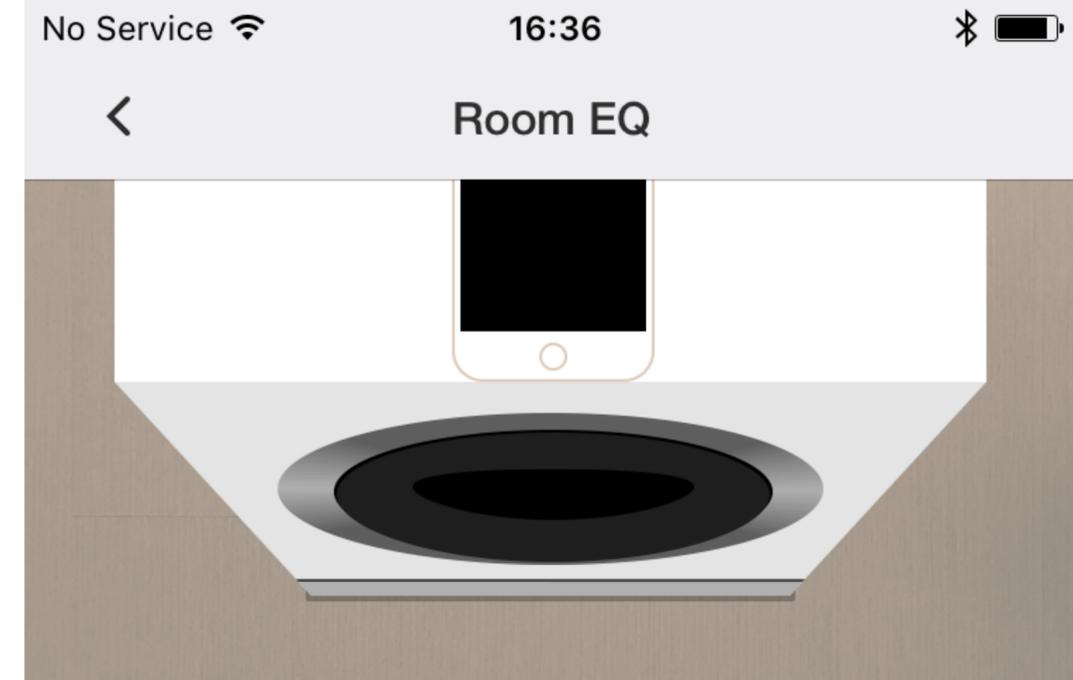
Place this device on top of the subwoofer with the bottom of it facing a side with a driver, as depicted above. Once you proceed, the subwoofer will emit a tone to use for calibration.
