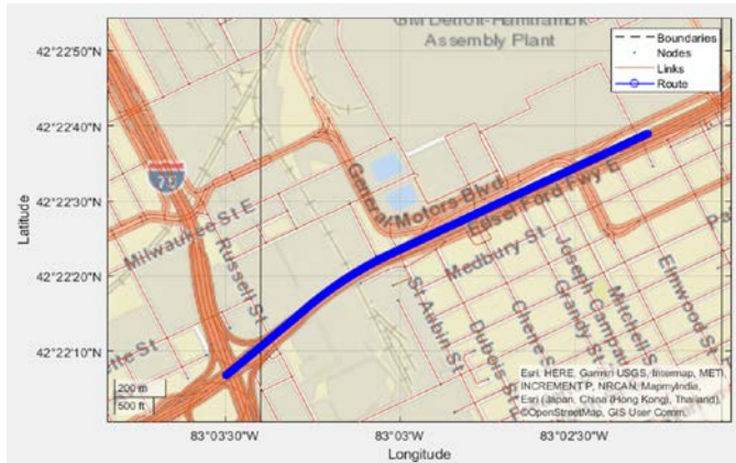
Figure 1. HD Map and driving route with recorded GPS data
