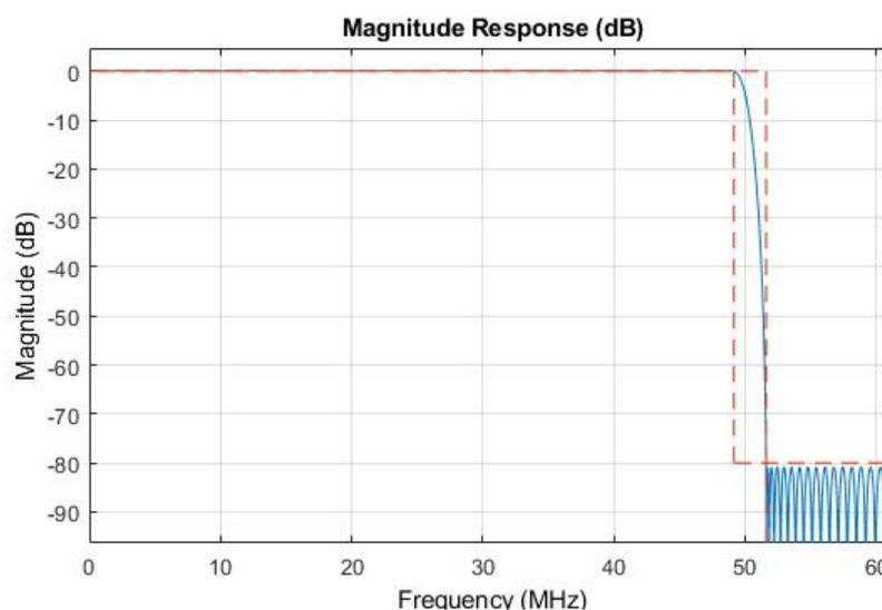
Figure 6. Magnitude of the filter response for the NR-FR1-TM3.1a waveform.
