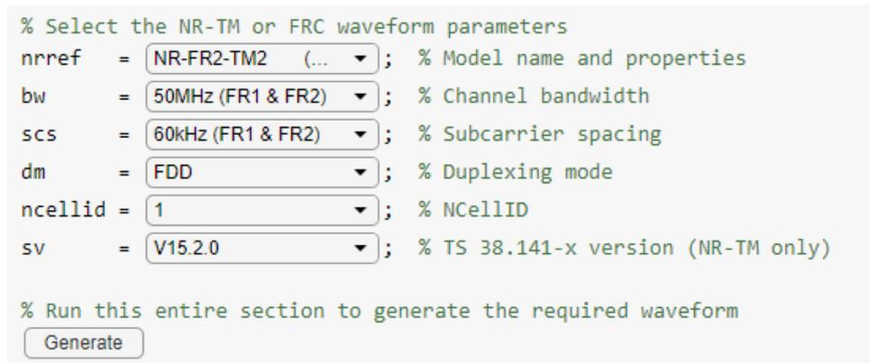
Figure 1. Selecting parameters for an NR-FR2-TM2 waveform.
